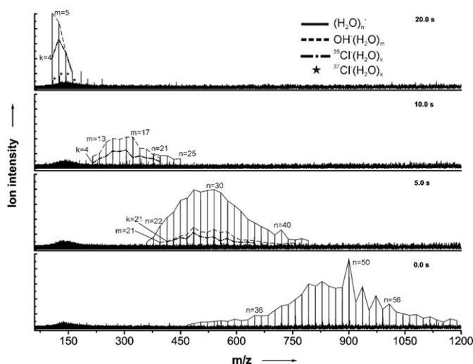
**Fig. 1.** Selected mass spectra for the reaction of  $(\text{H}_2\text{O})_n^-$ ,  $n = 30\text{--}65$ , with  $\text{C}_6\text{H}_5\text{Cl}$  at a pressure of  $7.7 \times 10^{-9}$  mbar, after 0 s, 5 s, 10 s, and 20 s. For  $n < 30$ ,  $(\text{H}_2\text{O})_n^-$  detach electrons in parallel to the black-body radiation and collision induced evaporation of water molecules, explaining the poor signal-to-noise ratio in the 10 s spectrum.
