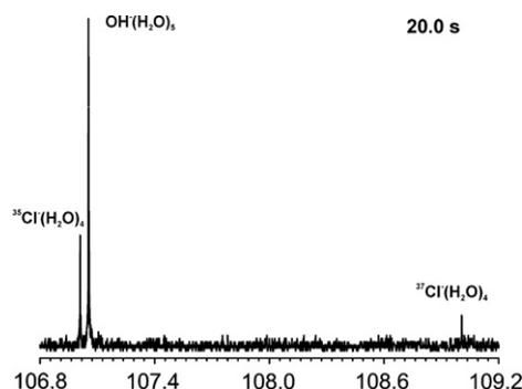
**Fig. 3.** Most intense peak group after 20 s.  $\text{OH}^-(\text{H}_2\text{O})_5$  and  $^{35}\text{Cl}^-(\text{H}_2\text{O})_4$  are two distinct peaks in this mass range.  $^{37}\text{Cl}^-(\text{H}_2\text{O})_4$  is present corresponding to the natural abundance of the heavier chlorine isotope.
