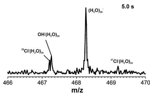
**Fig. 2.** Peak group around  $(\text{H}_2\text{O})_{26}^-$  after a reaction delay of 5.0 s. The hydrogen transfer product  $\text{OH}^-(\text{H}_2\text{O})_{25}$  indicates that the Birch reduction of chlorobenzene towards  $\text{C}_6\text{H}_5\text{Cl}$  has taken place. It is resolved from the isobaric peak of  $^{35}\text{Cl}^-(\text{H}_2\text{O})_{24}$ .
